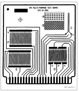
Figure 1 IPC-B-25A Test Board
