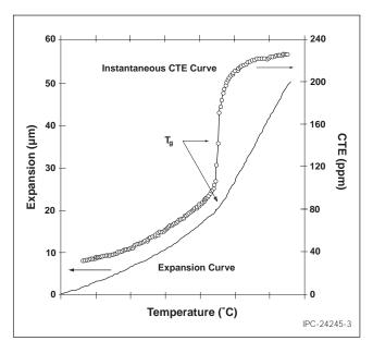
Figure 3 TMA Expansion Curve and Instantaneous CTE Curve
