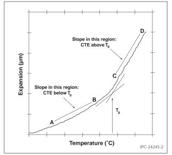
Figure 2 TMA Expansion Curve
