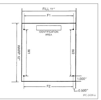
Figure 1 All dimensions are in inches. Four measurements are required as indicated. Locate measuring points approximately 12.7mm [0.500 in] from each edge in the fill direction, and 25.4 mm [1.00 in] from each edge in the warp direction.
