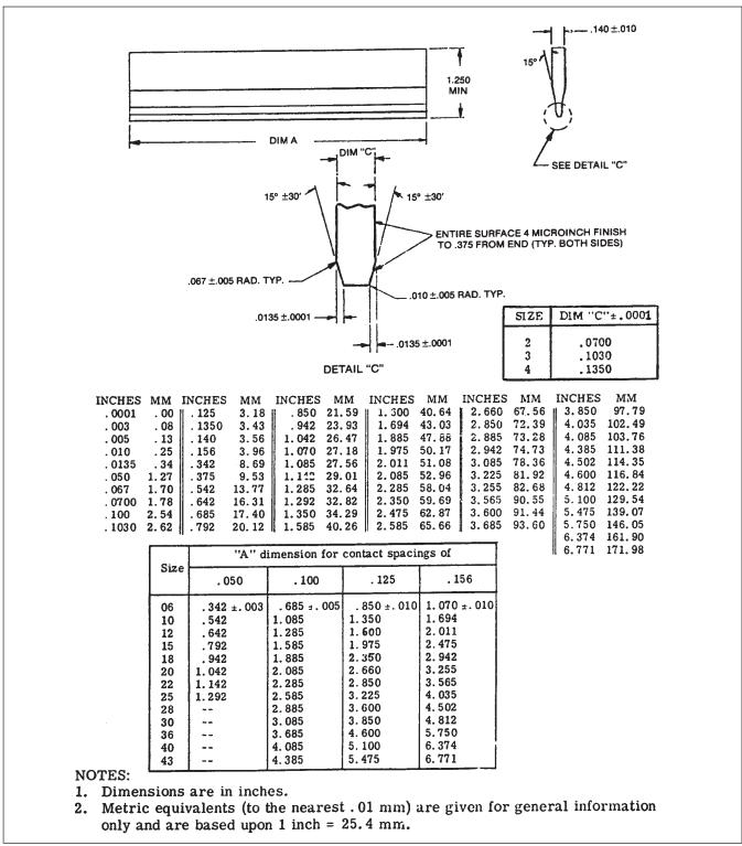
Figure 1 One Piece Edge Connector Mechanical Gages
